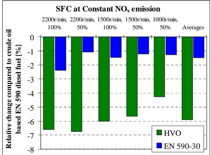
Figure 8. Engine smoke (FSN) and specific fuel consumption (SFC) when NO<sub>x</sub> is equal with all fuels.
