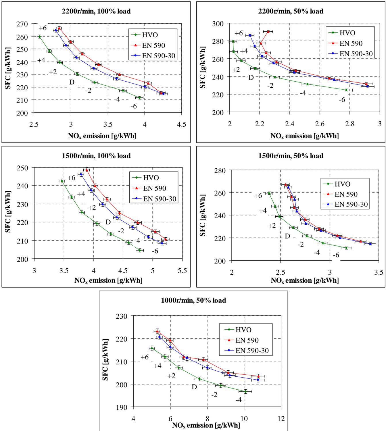
Figure 6. Trade-off between NO<sub>x</sub> and specific fuel consumption (SFC). "D" means the default main injection timing. + or - sign and the number means a start of main injection in °CA after or before the default setting.
