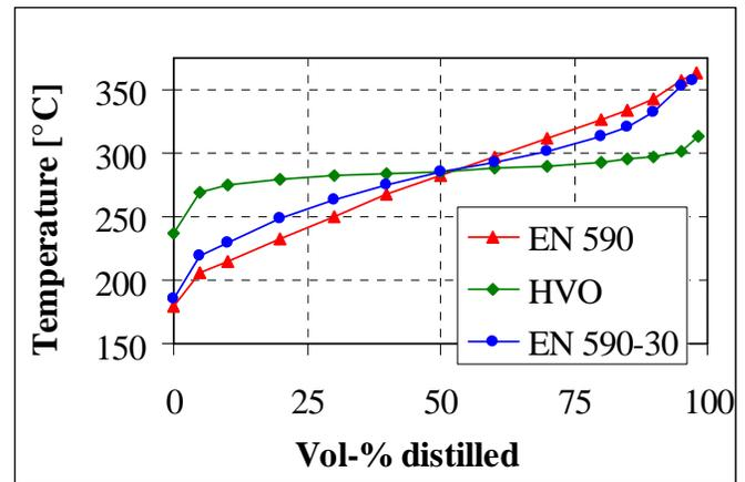
Figure 3. Distillation curves of the test fuels.
