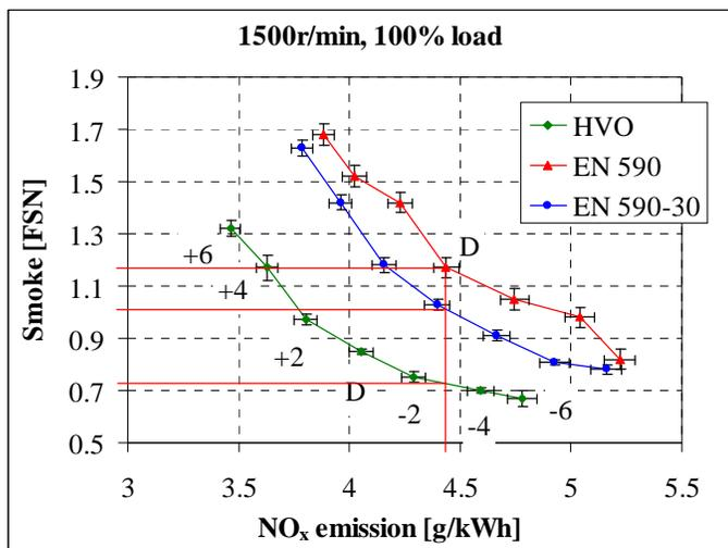
Figure 7. Example how smoke is obtained when NO<sub>x</sub> is considered equal between the test fuels.
