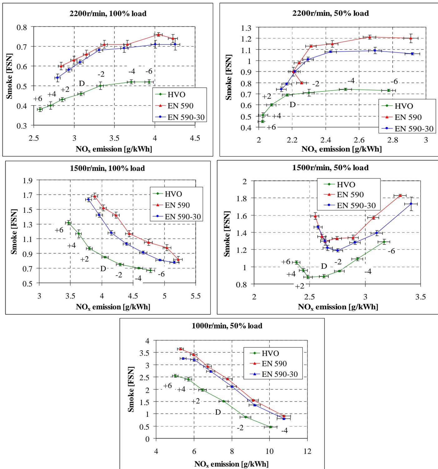
Figure 5. Trade-off between NO<sub>x</sub> and smoke. "D" means the default main injection timing. + or - sign and a number means the start of main injection in °CA after or before the default setting.
